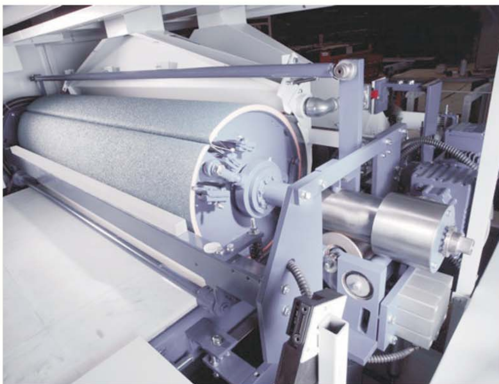
The deburring cylinder with a diameter of 420 mm is so soft, that it covers the edges of the sheet metal parts and therefore grinds with more pressure in these areas.
