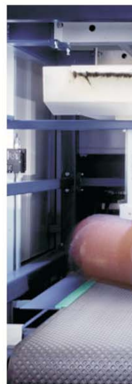
The deburring cylinder with a diameter of 420 mm is so soft, that it covers the edges of the sheet metal parts and therefore grinds with more pressure in these areas.
