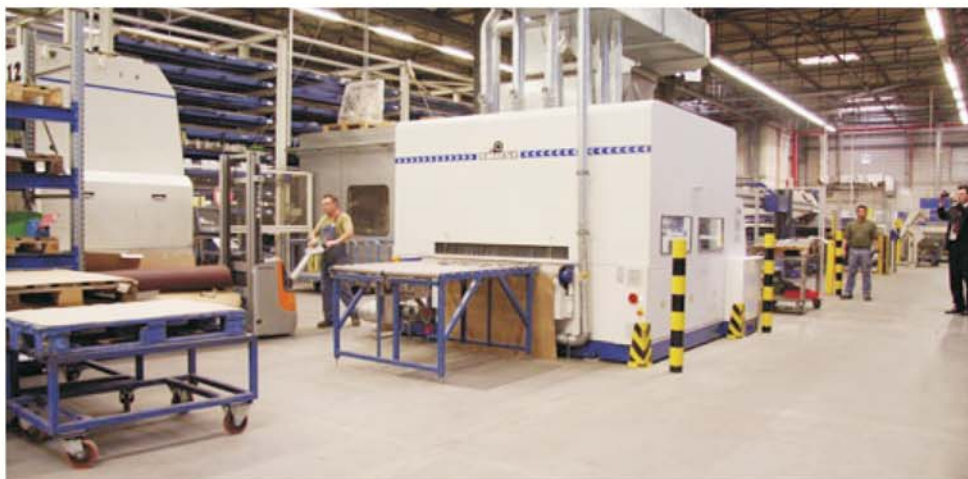
Where before two machines were needed, today one is sufficient. The EG M/ Rotation by Ernst combines deburring cylinder and rotor head with abrasive lamella brushes.
