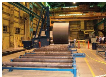
Figure 5 A feed table with staggered rollers and lateral alignment cylinders positions nonrectangular plate as it is rolled into a slightly conical section.
