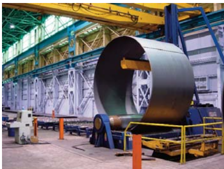
Figure 4 A support beam positioned above the roll set can prevent the rolled section from distorting, especially when working with thinner material.
